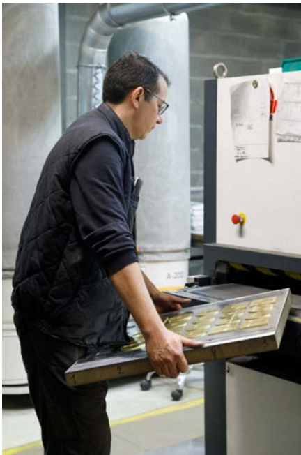
Sandblasting of Luce lighting plates, Paris, France.
